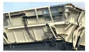
Hydraulic folding hopper extensions allows for increased capacity. Quick and easy set-up from ground level in a matter of minutes (Optional)
