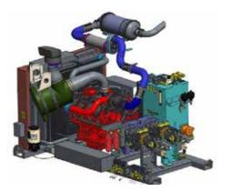
A powerful Scania engine with a low operating speed combined with an efficient hydrostatic drive creates a very responsive shredding action with protection against unshreddable contaminants
