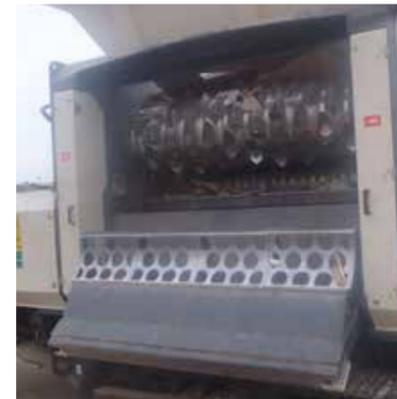
Medium speed shredder with aggressive cutting teeth
