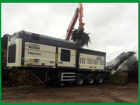
The TSS 390's 3m long shredding shaft was expertly designed in-house and is made from heavy-duty steel, with easily replaceable, bolt-on shredding teeth. Being hydrostatically driven, it offers the benefit of full speed reverse, as well as protection against contaminants. Customisable shredding programs enable the operator to configure the machine to their specific requirements and offers improved shaft cleaning in difficult applications, reducing wrappage and optimising throughput.
