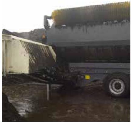
Double sided unrestricted drum access via two large swing out doors allows for easy maintenance and cleaning
