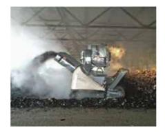
Both indoors or outdoors: The TWT 500 is an all-rounder being able to stack triangular and trapezoidal windrows in such a way that 30% of space can be saved.
