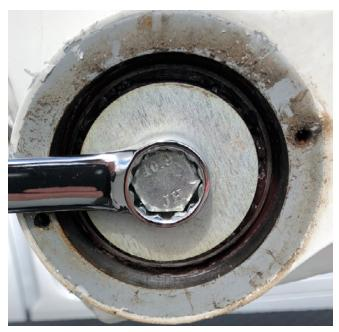
Use two wrenches, one on each side of the roller shaft. The bolts have thread locker on them. Remove a bolt from the shaft and slide out the shaft away from the rollers and shims. The shims are located between the cone bearing and spacer.
