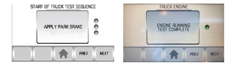
During some steps, a function button will appear on Button 1. This button will perform a walk-through of multiple functions such as: checking the park brake, making sure the engine is running, verifying the PTO, start/stop, throttle and light operations.
