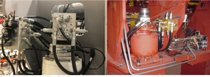
Planetary Slip Drive Test & Adjustment
