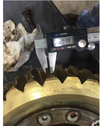
If no cracks are found and the gear shows minimum wear, it may be reinstalled as is. If the thickness is less than .054, rotate the gear on the shaft 180 degrees.
