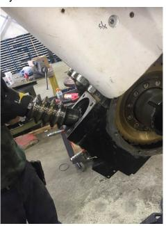
**STEP 16**Install the bearing race and machine bushing into the gearbox.
