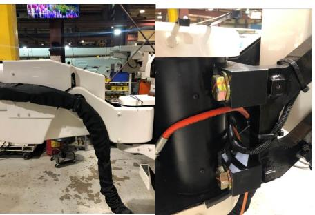
Using the upper controls, move the upper boom away from the boom tip assembly and retract the boom until it is in a comfortable position to disassemble the leveling gear box.
