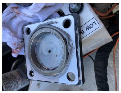
Reinstall the end plate and torque to 170 ft-lbs. with red Loctite.
