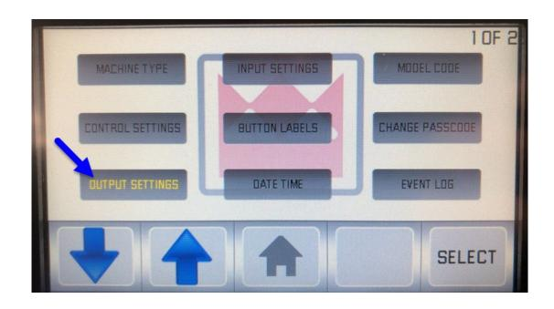
Use the up/down arrow to choose the output the component is wired in to. Press the Select button and scroll until the correct button is selected. Press the Select button again to lock in the output and the chosen button.
