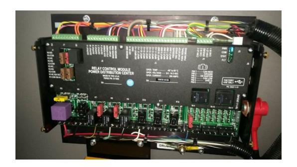
There is a wide range of components and accessories that can be wired into the switch panel. The limitation on what can be wired into the switch board is the amperage requirements. The output limitations are shown below:
