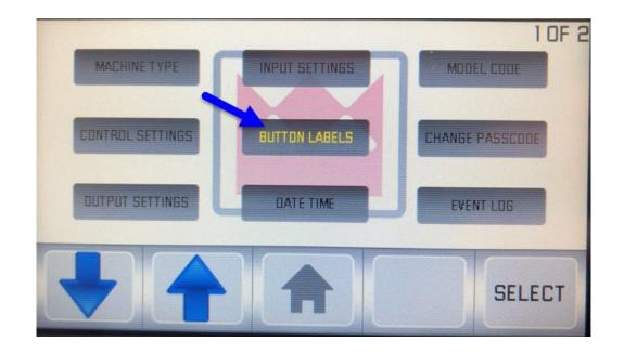
Use the up/down arrow to scroll through the buttons until a spare button is highlighted. Push the Select button and scroll through the options to find the best description for the installed component. Once the description is found, press the Select button.
