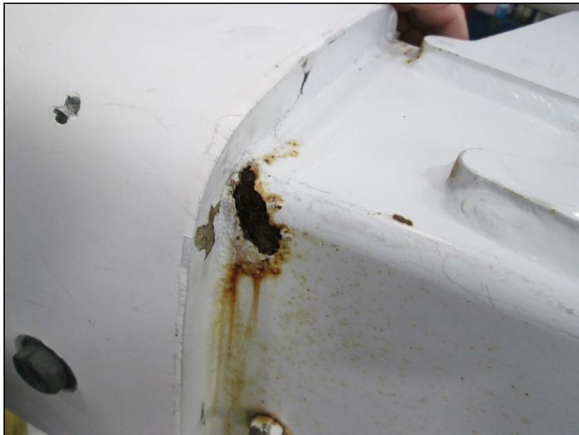
Water entering where the fiberglass is bonded to the steel can carry substances which can accelerate corrosion of the steel. In cold climates, it can freeze and cause the bond to fail.
