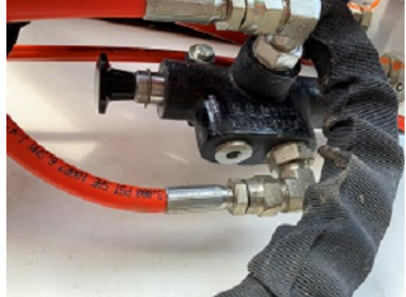
FIGURE 2 - Push/pull style selector valve
