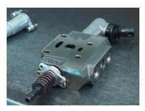
Remove the seal retaining flanges or lever boxes (Handles).
