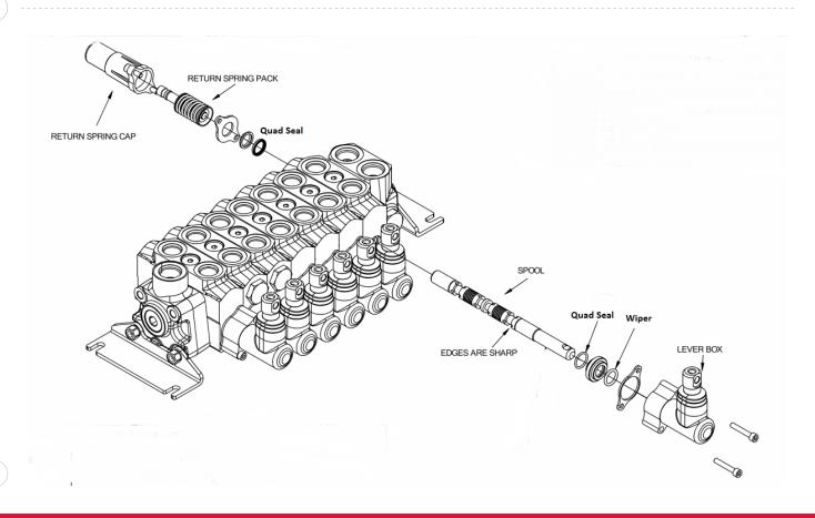
Remove the old flanges, wipers and O-rings from both ends of the spool.
