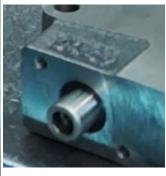
Install the return springs, you will need to hold the spools that are controlled by the single stick from turning while torquing the return springs to 4.43 ft-lbs. (53 in-lbs.).
