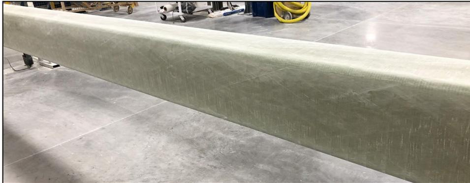
**Note:** Do not handle the sanded boom with bare hands since the oils and salts from the skin will contaminate the boom surface, preventing adherence of the coating. The boom can only be handled with clean gloves in this condition.
