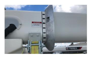
**STEP 3**Remove the orange bonding cables to the single stick at the boom tip.
