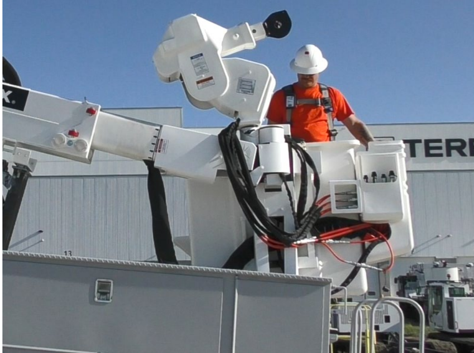
Platform not level with unit
