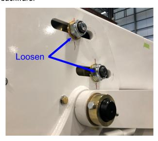
Do Not remove the nuts or back them off to the point that the nylock is removed from the threads. If the nuts are removed or the nylock disengages the threads the nuts must be replaced. If new nuts are installed lubricate the threads with anti-seize, Terex part number 65370833.
