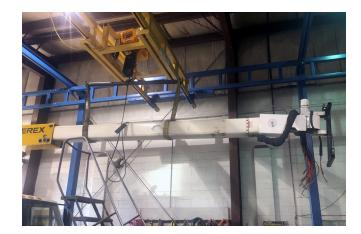
Place fiberglass section on supports rated for the load.
