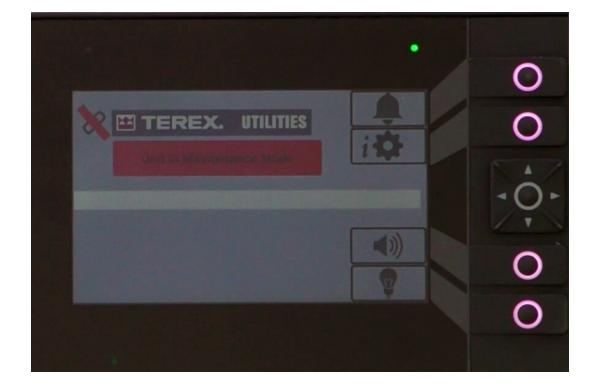
With a level verify the lower boom is level, then push and hold the Zero Lower Boom button.
