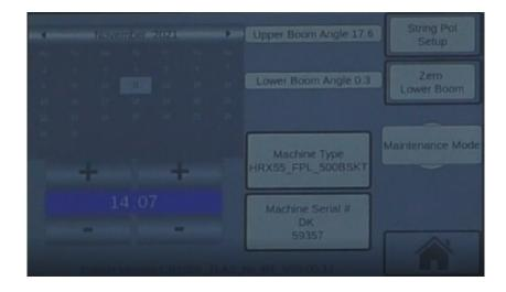
To zero out the angle sensors, push on the display where it says Maintenance Mode. The button will turn green indicating the system is in maintenance mode. This mode will prevent any alerts from being sent out while testing.
