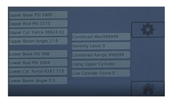
The Combined Max is what is allowed by the load chart depending on the boom angles. In this example, the max is showing 999999 because at this boom angle (lower at 0.3) there is no capacity per the load chart.
