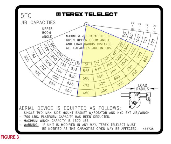
The load radius is 3.5 feet. Based on this load radius, we will be using the 3rd band in the loadchart for a radius of 3' to 4'.
