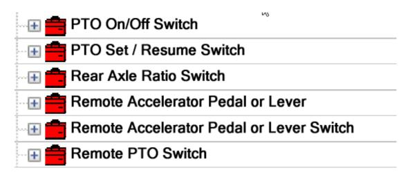
For all diggers and aerials, should have Remote PTO switch enabled and source address set to 121.
