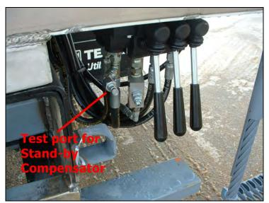
If the standby pressure needs adjustment, go to the pump and locate the adjustment (Reference the pictures on the next page for location). Remove the Allen head plug with a 5/32" Allen wrench and then use a 1/4" Allen wrench to adjust the pressure. When standby pressure is set correctly reinstall the plug.
