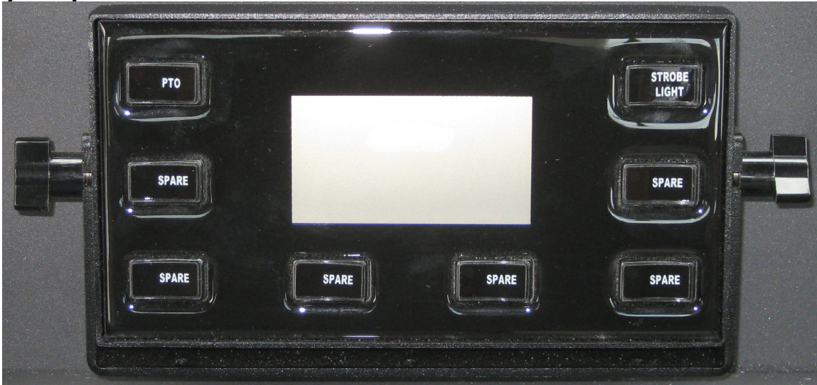
FIGURE 8 - Switch and display panel, usually with 8 switches
