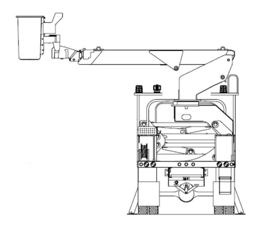
Attach a dynamometer between the boom tip and the load line for pulling up the boom (negative deflection).
