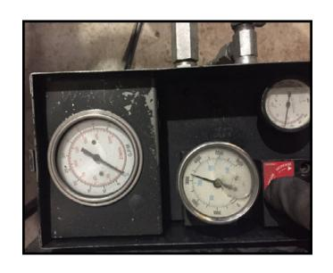
Slowly increase the pressure again, while watching the flowmeter. The flow should stay at the recorded flow or no less than 80% (15.2 gpm for 19 gpm and 16.8 for 21 gpm) of the flow until the pressure is within 250-300 psi of the compensator setting. If it is less than that, then the pump is bad.
