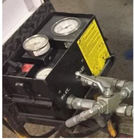
To connect the large side of the pump to the flowmeter, hook up the inlet hose to the hose coming from the Outrigger/Unit selector valve. Use the selector as a shut-off valve to stop oil from dripping.
