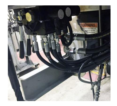
Connect the return line to the tool return quick coupler at the tail shelf.
