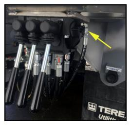
**STEP 4**Hook the load sense line up to the tee on the inlet side of the flow control.
