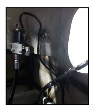
The small pump is a pressure compensated pump. Hook up the pressure line to the hose going to the flowmeter.
