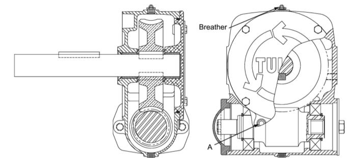
NOTE: Oil should be level with the bottom of the check/fill plug (A) when the winch is at the position shown. Maximum 120 hour interval.
