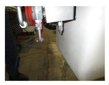
Elevate the platform to at least 4 feet above the ground. Visually check that all jumpers, the voltage source from the dielectric tester, and the return are still connected once the unit is in position.
