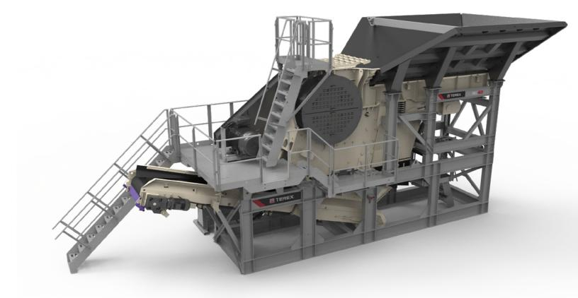
It features the Terex® TJ2844R single toggle jaw crusher with hydraulic overload protection as standard. It has a fully galvanized steel structure including walkways, steps, guardrails and product conveyor and is CE compliant.
