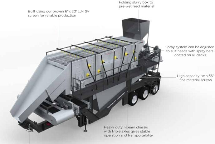
Designed with portability in mind, easy on/off landing jacks help reduce set up time
