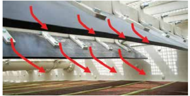
Optional deflector plates increase bottom deck effective area and capacity
