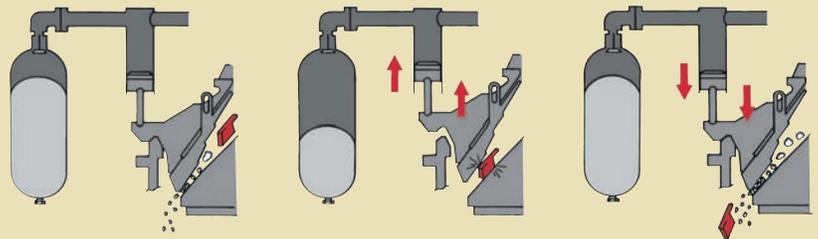
a nitrogen gas bladder in the accumulator. Once the crushing cavity is cleared, the gas forces the oil back into the relief cylinder and the bonnet lowers to its original position.
