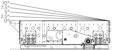
TSV screen installs from 0° up to 10° in 2.5° increments
