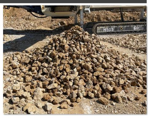
Location: POLAND Machine: MDS M515 Application: STICKY MATERIAL / LIMESTONE Throughput: 450-500 TPH, Fuel Efficiency 15 L/hr
