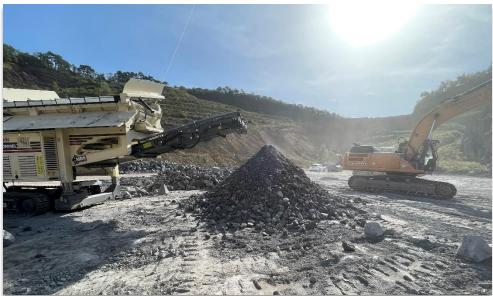
Location: GERMANY Machine: MDS M515 Application: PROCESSING RIP-RAP Throughput: 450-500 TPH, Fuel Efficiency, 15 L/hr
