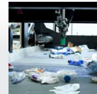
Fast Picker Robotic Sorting
