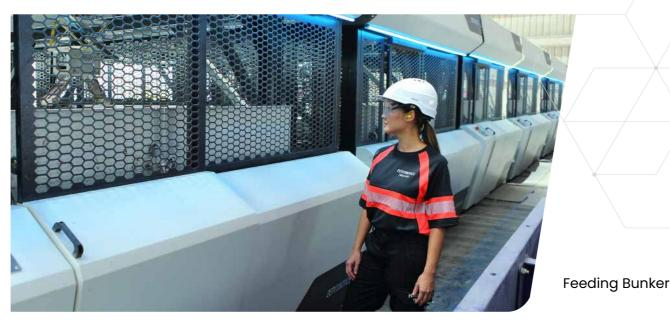
The Heavy Picker can sort several high-purity fractions, weighing up to 40kg, simultaneously with the help of heavy-duty arms and high IQ artificial intelligence.
